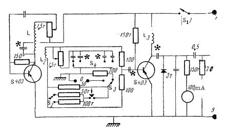
Fig. 1. Circuit of the semiconductor rheograph. The components marked by an asterisk are adjusted when tuning the instrument.
